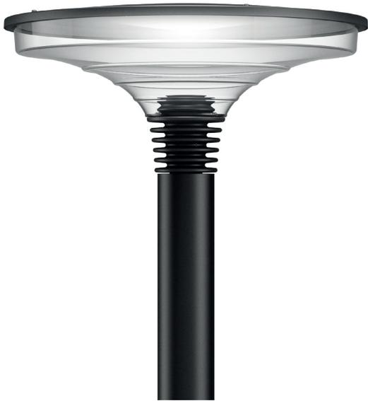
**BECCO** is born with LED and many necessary components are integrated parts of the luminaire design. The heat sink forms a characteristic connection between the column or bollard and the lantern, and it is the base of the LED module as well. The light source is not visible, and the indirect, non-glaring light is spread by means of the arched roof plate.
